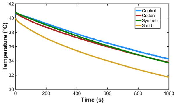
**Figure 7:** Temperature at the bottom surface of the block as a function of time with wind speed of 3.2 m/s. Note the initial temperatures are different, so direct comparisons are difficult to make from this graph.
