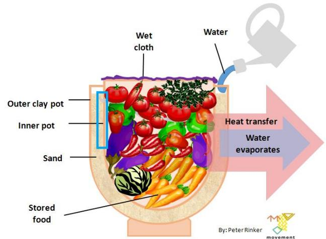
**Figure 3:** Cartoon cross section of a pot-in-pot refrigerator (6). Water is poured into the sand between the two pots and evaporates through the outer pot, cooling the food in the inner pot. The blue box marks the portion of the device analogous to the experimental setup.
