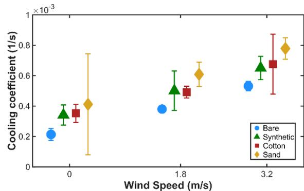
**Figure 10:** Cooling coefficients plotted as a function of wind speed and the markers organized by material type. The data points are staggered at each wind speed to improve readability.
