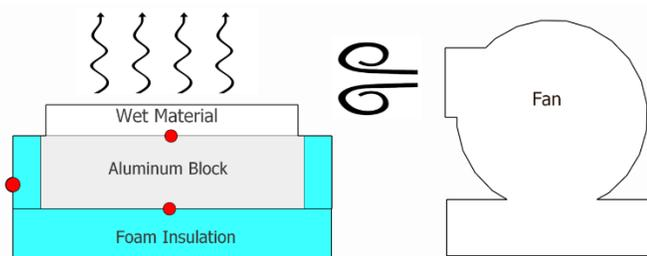
**Figure 6:** Schematic of experimental setup with a fan blowing over the water-soaked material. Temperature sensors (red dots) are placed to record the temperature at the top and bottom of the block and the ambient air. These are connected to Logger Pro data collection units (not pictured).
