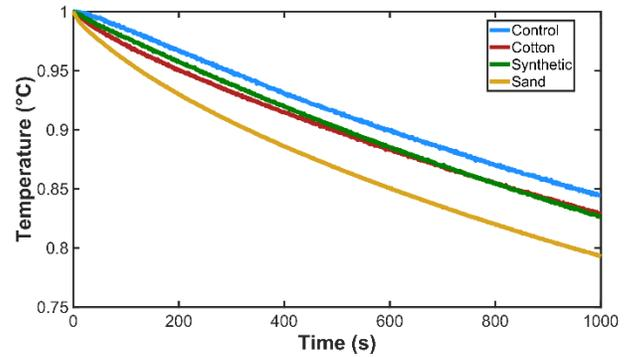
**Figure 8:** Ratio of temperature at time  $t$  to initial temperature over the data collection period. Note the improved cooling by placing a wet material on the block.
